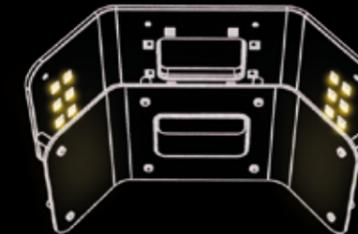
MDP2 with central LEDs at full power + polarizing filter, lateral LEDs off
