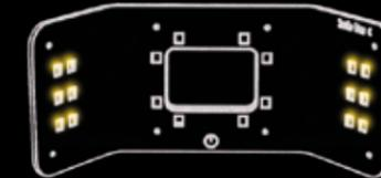
MDP2 with lateral LEDs at full power + diffuser, central LEDs off
